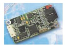
3M MicroTouch EX II Series controllers bring flexibility and feature-rich functionality to capacitive and resistive touch screen applications. This high performance electronics platform is based on the innovative MicroTouch EX II ASIC, designed to provide higher resolution touch coordinates, on-chip RAM, and a wider operating temperature range.
